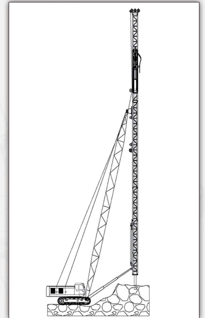
APE HYD. IMPACT HAMMER DRIVING 24" SQUARE CONCRETE
